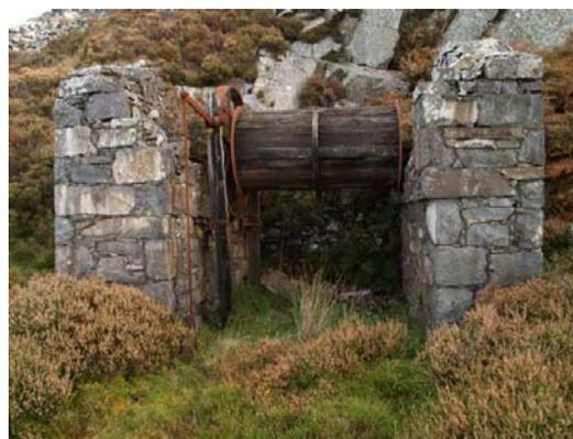
**Incline winding drum from Tan Y Graig quarry, brake mechanism on the left end of the drum**
