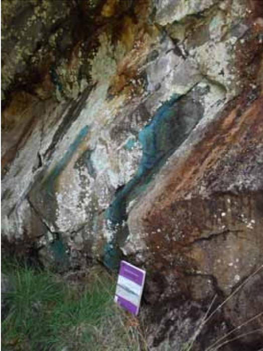
*“A partly filled trial level....blue secondary copper minerals staining the walls of the excavation show that the rock contains chalcopyrite”*
