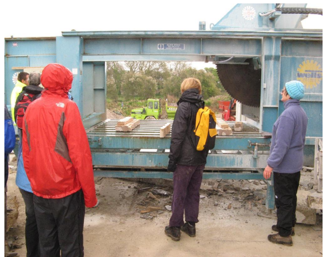
The large diamond saw apparatus used for cutting the limestone blocks to size in the yard at Anglesey Masonry.
